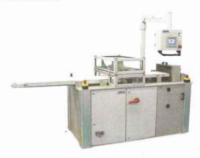
AZCO Corporation has designed a precision single surface indexing system for feeding and cutting flexible materials to length. This is ideal for applications where material can only be contacted on one side. A unique vacuum transfer system is controlled by a servo motor. For reliable clean cuts, a SUR-CUT modular knife assembly cuts the material to a high accuracy of +/-0.01".
